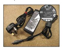
Technically designated as FELV (Functional Extra Low Voltage) (ITE = Information Technology Equipment) PSUs these devices internally have a double-insulated PSU that provides a low output DC voltage. The mains supply earth is connected to the low voltage negative of the DC output via typically by a 10 to 100 ohm resistor. As these PSUs have an 'earth' manufacturers are unable to place a double-insulated symbol on the product.
